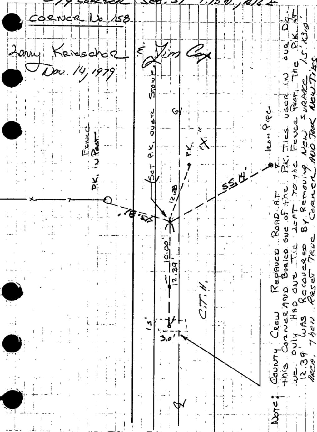
**Note:** County Crew Repaved Road at this corner and buried one of the P.K. Ties used in our Dig. We only had one tie left to the fence post, the P.K. at 12.39' was recovered by removing new surface 15' x 30' area. Then reset the corner and took new ties.
