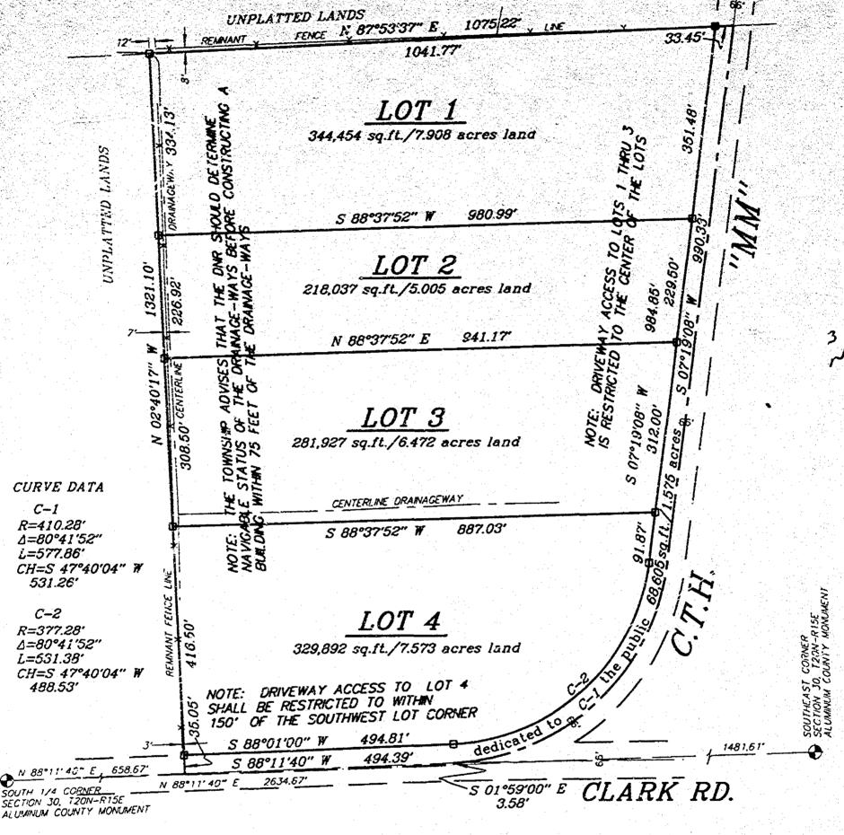
BEARINGS ARE REFERENCED TO THE SOUTH LINE OF THE SOUTHEAST 1/4 OF SECTION 30 T2CN-R15E, ASSUMED TO BEAR: N 88°11'40" E
