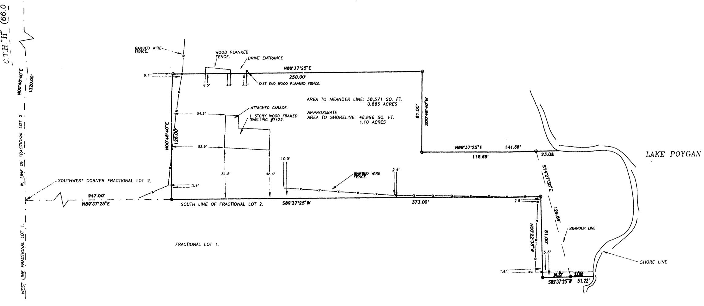
• DENOTES 3/4" X 24" IRON RODS SET, WEIGHING NOT LESS THAN 1.50 LBS PER LINEAL FOOT. ALL DISTANCES ARE MEASURED TO THE NEAREST HUNDREDTH OF A FOOT.
