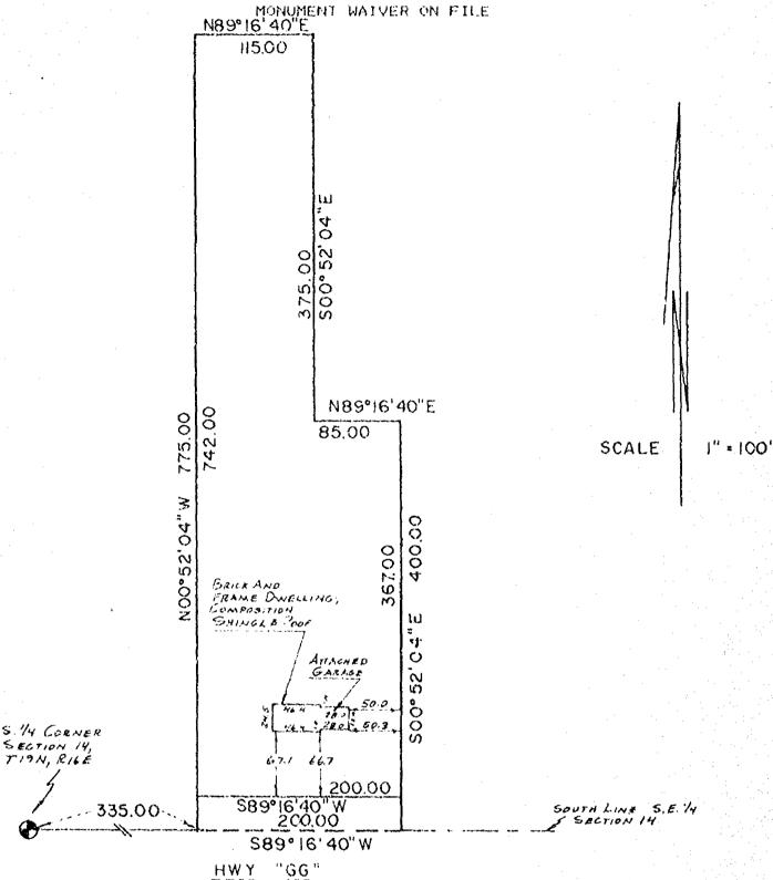
I Certify that I have surveyed the above described property (Property), and the above map is a true representation thereof and shows the size and location of the Property, its exterior boundaries, the location and dimensions of all visible structures thereon, boundary, fonces, apparent easements and roadways and visible encroachments, if any.
