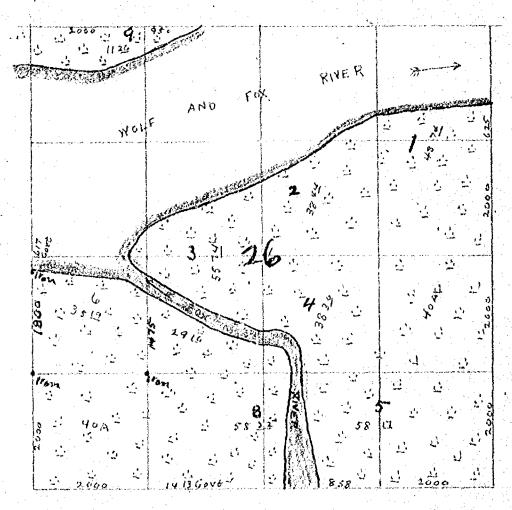
I Began at a iron stake set at the corner of Sec 27-28-33-34 Ran East 80.00 chs V 3-10' I then turned North at Right angles and surveyed out not 6 or NW 1/4 SW 1/4 Sec 26 and set iron stakes as shown marked in Red Ink on above map stakes set was 4 inch Boiler flue marked with cold chissel 12 ft long Drove in the marsh 10 ft 2 ft out of ground with figures in plain wight Began Feb 28th Completed March 1st 1918
