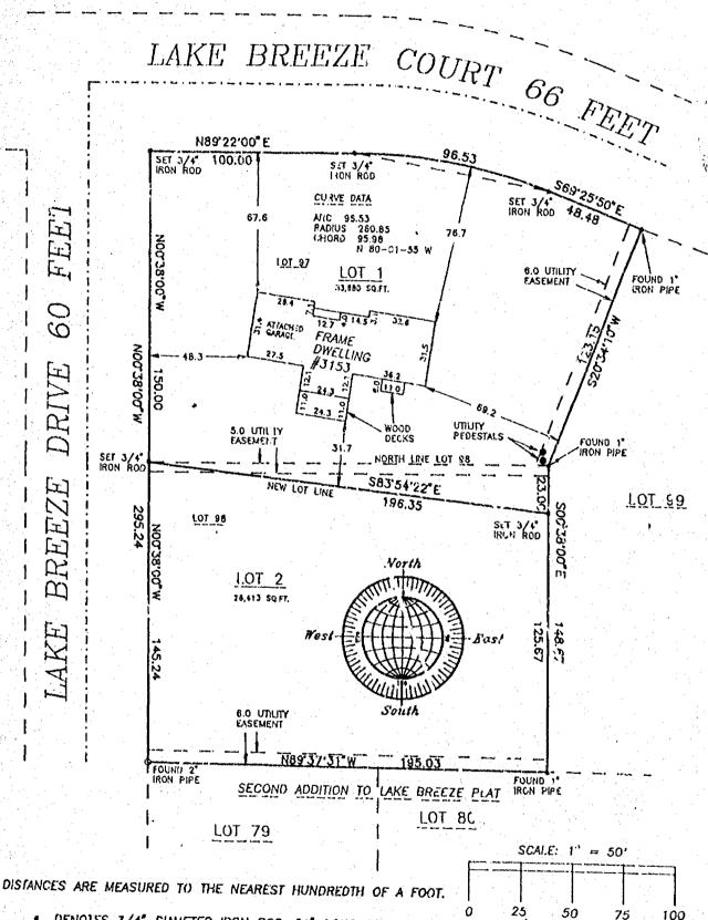
DENOISS 3/4" DIAMETER IRON ROD, 24" LONG, V NOT LESS THAN 1.13 LBS PER LINEAL FOOT SET.
