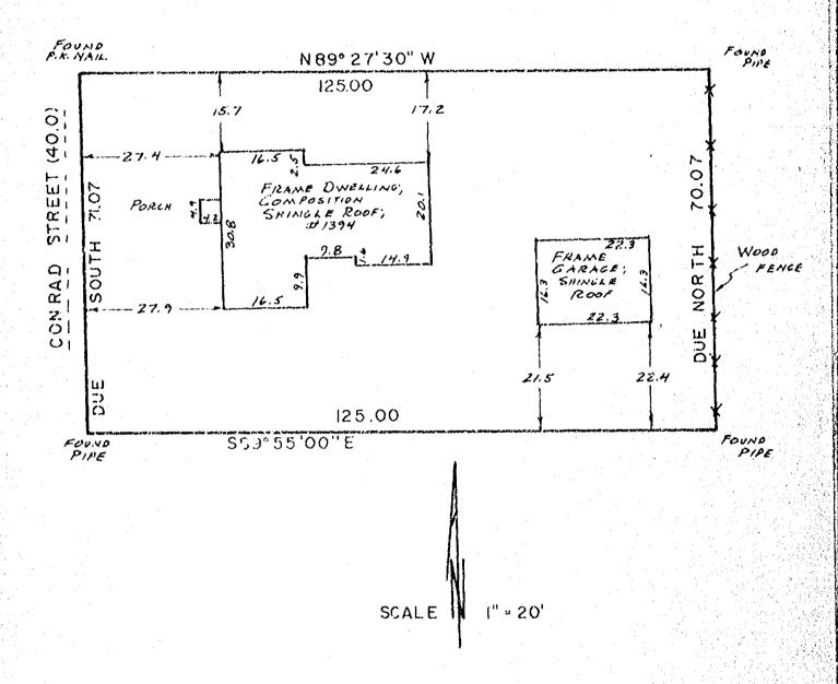
Certify that I have surveyed the above described property (Property), and the above map is a true representation thereof and shows the size and location of the Property, its exterior boundaries, the location and dimensions of all visible structures thereon, boundary, fences, apparent easements and roadways and visible encroochments, if any Continuous of the property,
