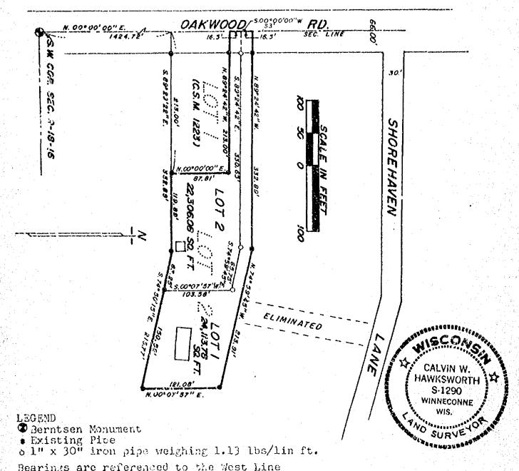
Bearings are referenced to the West Line of Sec. 9-18-16, assumed bearing N.00°00'00"E.
