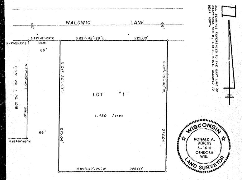
LEGEND 0 = 1"x 24" IRON PIPE WEIGHING 1.68 LBS / LINEAL FOOT SET. IRON PIPE FOUND. DATE: 9/24/84
