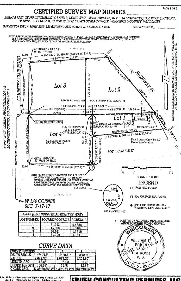
Note: WI Dept. of Transportation Right of Way maps for U. S. H. 43, dated 4/11/90 indicate that Curves 1. 2 & 3 are one curve with a centerline radius of 1.009.86 Pt., a length of 404.86 Pt. and a Delta angle of 12'08'45". This survey used this information and n atched it to curve information in CSM #2397,
