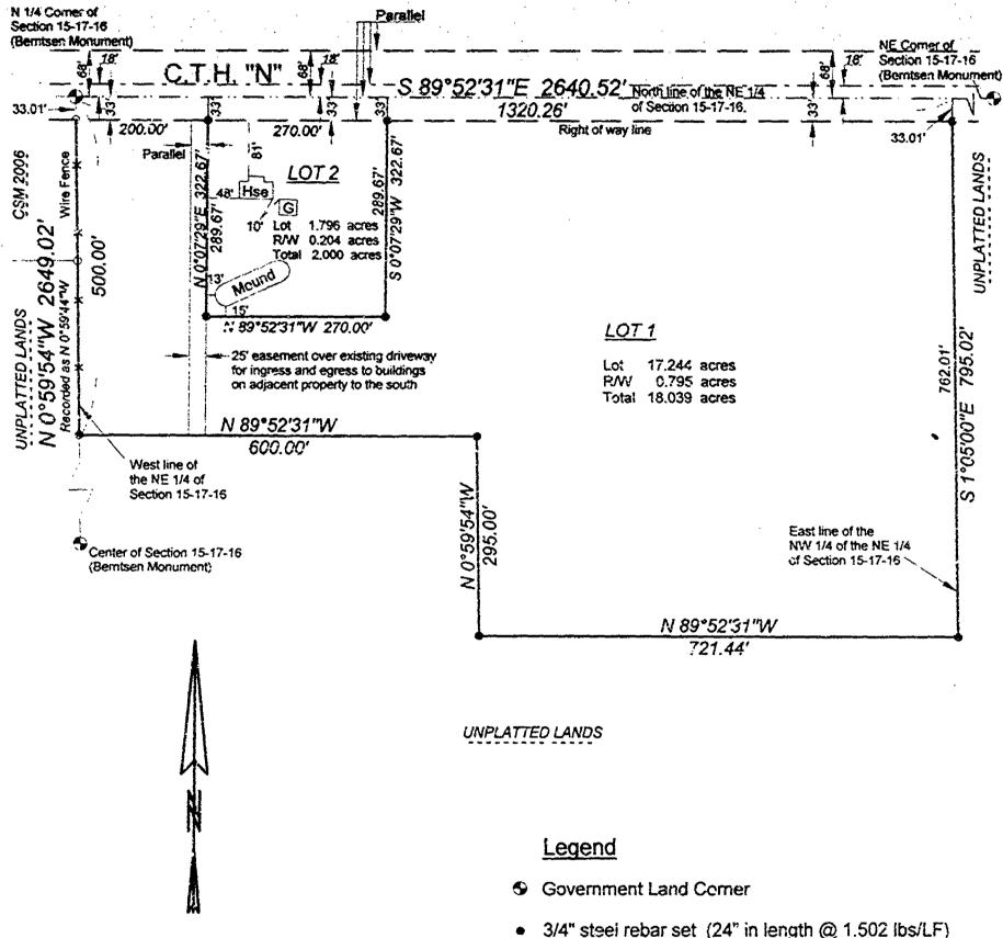
Bearings are referenced to the North line of the NE 1/4 of Section 15-17-16,
