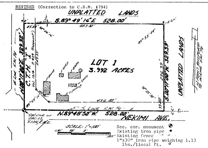
Bearings are referenced to the West line of the  $SW_4^1$  of Sec. 13, assumed bearing, NOO°17'00"E.
