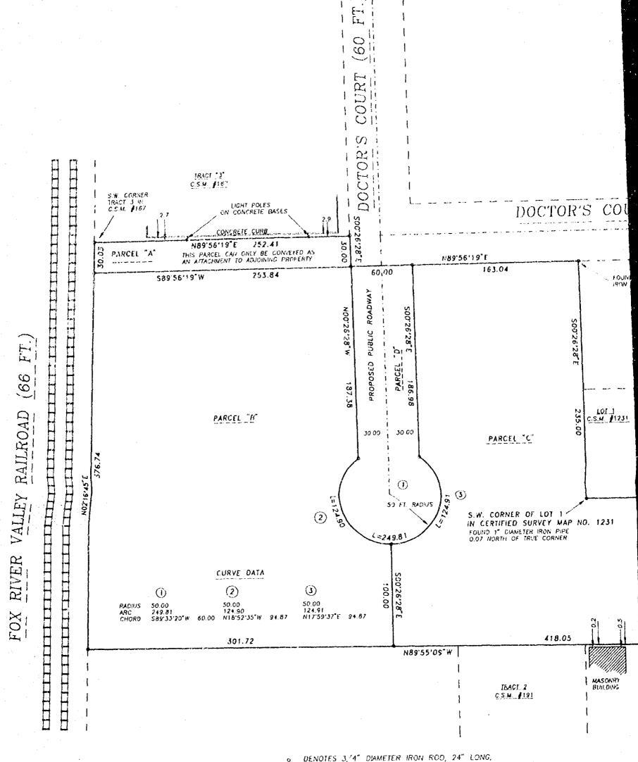
DENOTES 3,/4" DIAMETER IRON ROD, 24" LONG, WEIGHING NOT LESS THAN 1.13 LBS PER LINEAL FOOT SET.
