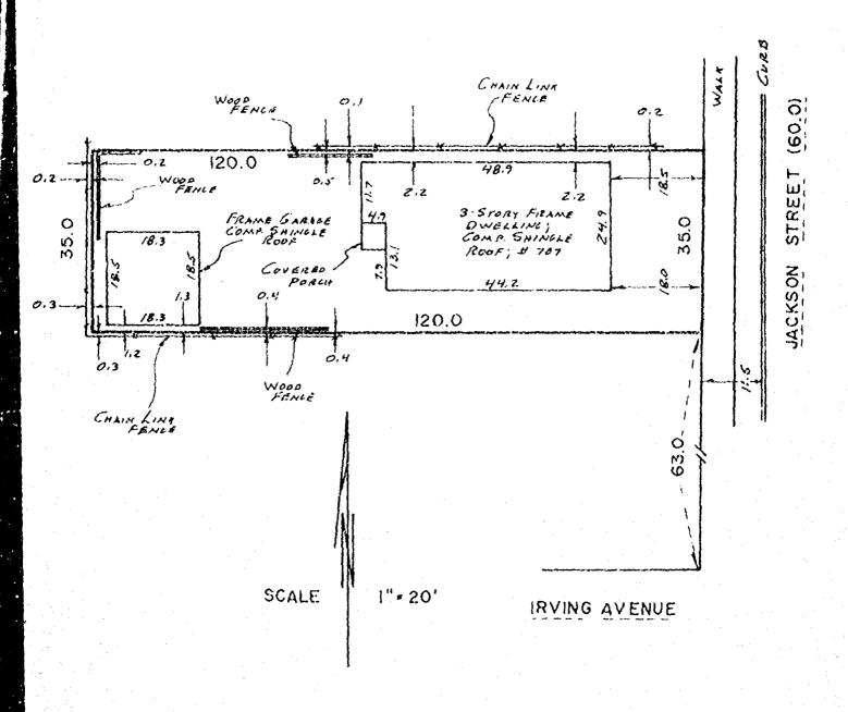
I Certify that I have surveyed the above described property (Property), and the above map is a true representation thereof and shows the size and location of the Property, its exterior boundaries, the location and dimensions of all visible structures thereon, boundary, fences, apparent easements and roudways and visible encreachments, if any,
