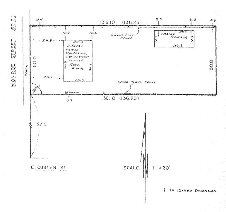
I Certify that I have surveyed the above described property (Property), and the above map is a true representation thereof and shows the size and location of the Property, its exterior boundaries, the location and dimensions of all visible structures thereon, boundary, fences, apparent easements and roadways and visible encroachments, if any.
