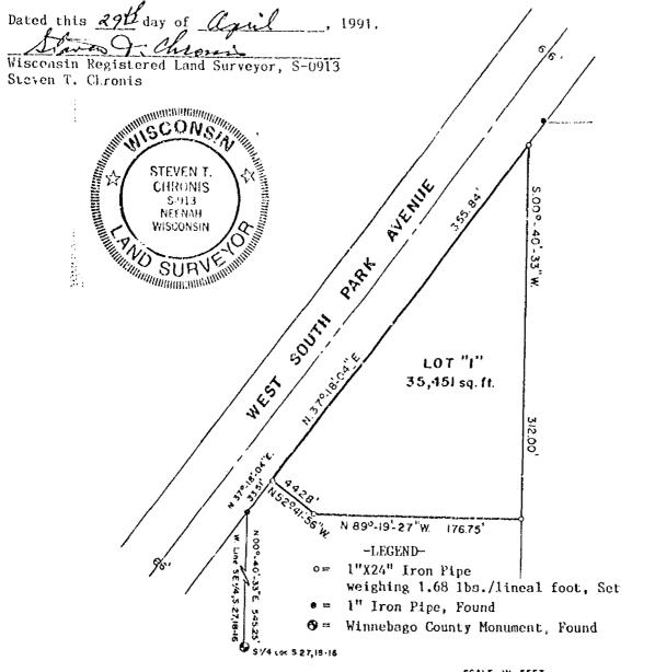
Bearings are referenced to the Weiline of the SEL, Section 27 Assigned N.00°-40'-33"E.
