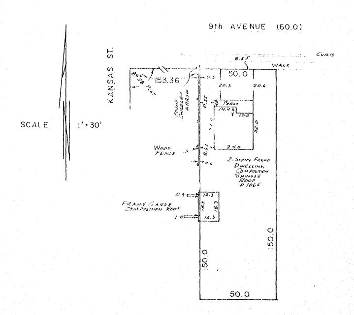
I Certify that I have surveyed the above described property (Property), and the above map is a trun representation thereof and shows the size and location of the Property, its exterior boundaries, the location and dimensions of all visible structures thereon, boundary, forces, apparent easements and roadways and visible encroachments, if any process of the present owners of the Property,
