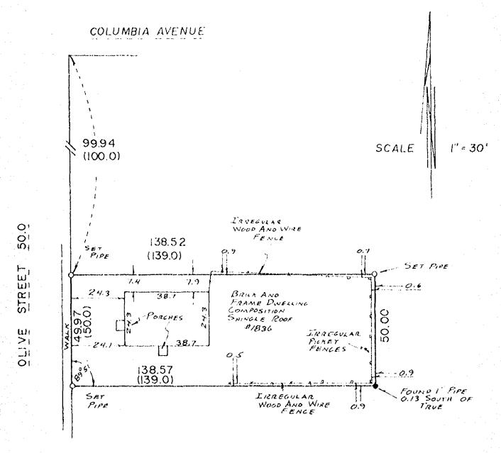
rentation thereof and shows the size and location of the Property, its exterior boundaries, the location and dimensions of all visible structures thereon, boundary, fences, apparent easements and roadways and visible encroachments, is apparent easements and roadways and visible encroachments, is apparent easements of the Property,
