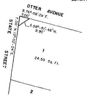
NOT E: NEW CORNERS TO BE SET AFTER PURCHASE, CORNERS WILL BE EITHER- I R 24" IRON PIPE OR CHISELED CROSSES IN CONCRETE.
