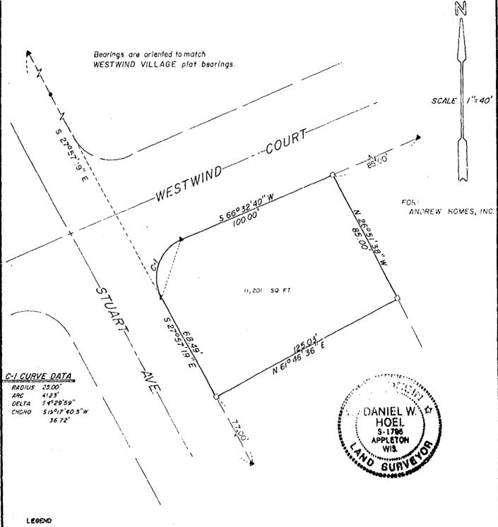
9/4"x 24" STEEL REBAR SET 15x 24" IRON PIPG SET 1-1/4"x 30" STEEL REBAR SET CHISELED "X" SET 9/4" REBAR FOUND 1" IRON PIPE FOUND 1-1/4" REBAR FOUND 2" IRON PIPE FOUND CHISELED "X" FOUND CHISELED "X" FOUND
