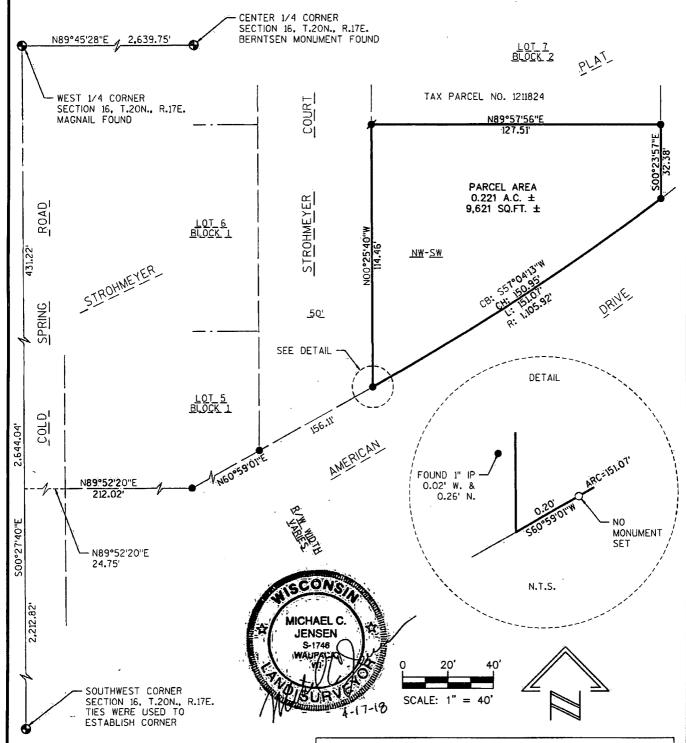
REFERENCE BEARING NORTH REFERENCED TO THE WEST LINE OF THE SW 1/4 OF SECTION 16,T.20N.,R.17E., WHICH BEARS SOO'27'40"E, BASED ON W.C.C.S. WINNEBAGO COUNTY
