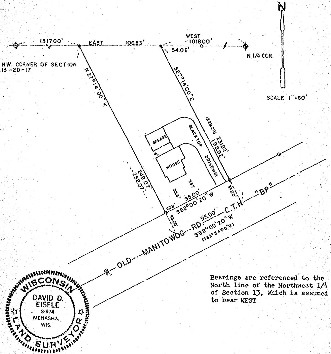
Bearings are referenced to the North line of the Northwest 1/4 of Section 13, which is assumed to bear WEST
