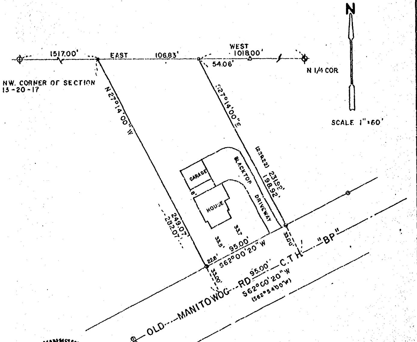
Bearings are referenced to the North line of the Northwest 1/4 of Section 13, which is assumed to bear WEST
