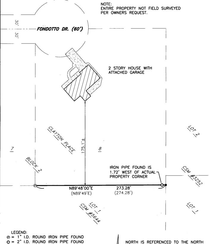
2" I.D. ROUND IRON PIPE FOUND 34" X 24" SOLID ROUND IRON REBAR SET, WEIGHING 1.502 LBS. PER LIN. FT.
