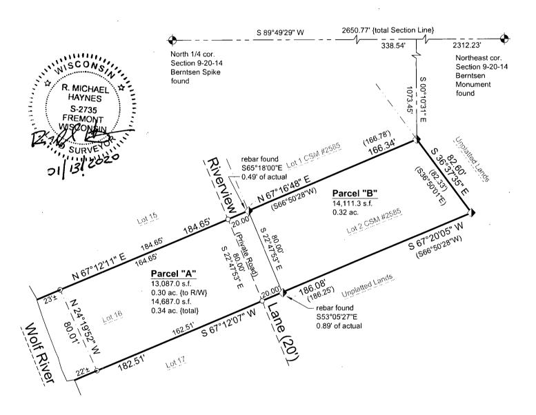
Bearings are referenced to the North line of the Northeast 1/4, referenced to bear S89°49'29"W
