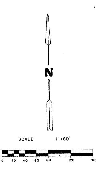
NOTE: ALL LINEAR MEASUREMENTS HAVE BEEN MADE TO THE NEAREST ONE HUNDREDTH OF A FOOT ALL ANGULAR MEASUREMENTS HAVE BEEN MADE TO THE NEAREST MINUTE AND COMPUTED TO THE NEAREST SECOND
