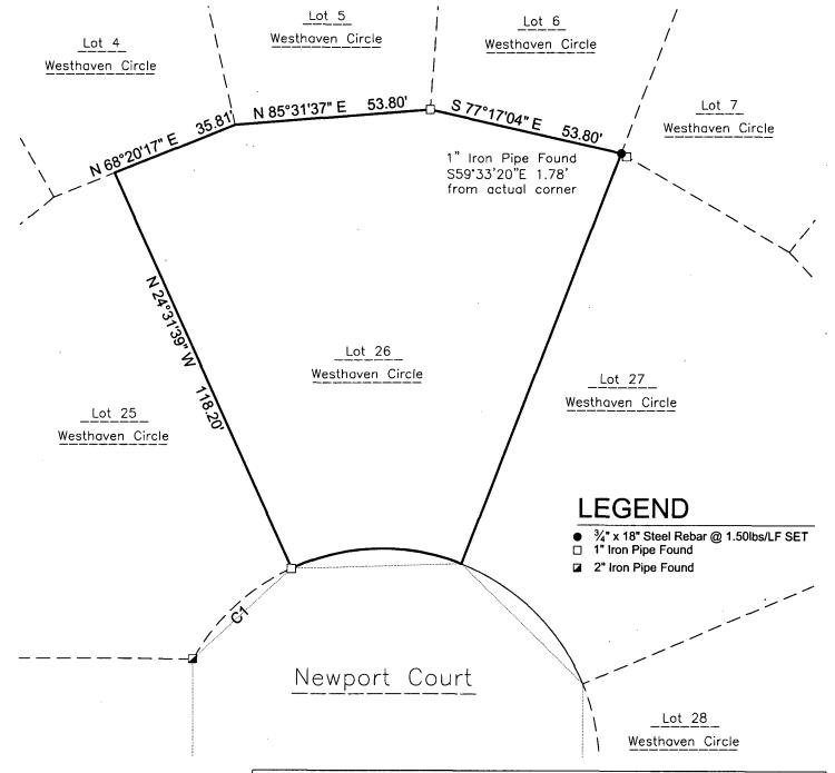
Note: Purpose to set Northeast Corner of Lot 26 due to disturbance of corner during construction activities.
