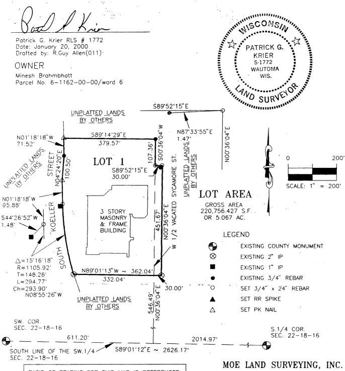
BASIS OF BEARING FOR THIS MAP IS REFERENCED TO THE SOUTH LINE OF THE SOUTHWEST QUARTER OF SECTION 22, T-18-N, R-16-E, WHICH IS ASSUMED TO BEAR S89'01'12"E.
