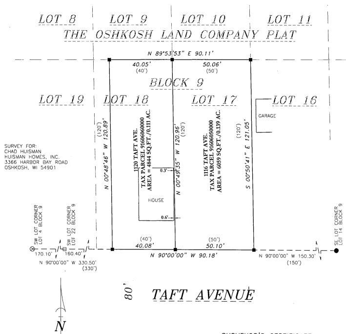
BEARINGS ARE REFERENCED TO THE NORTH RIGHT-OF-WAY LINE OF TAFT STREET ASSUMED TO BEAR N 90°00''' W
